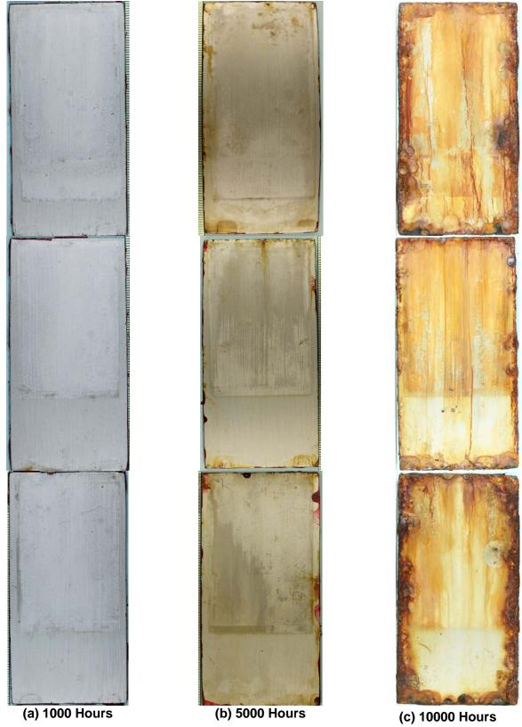
Figure 1. Images of the Three RUST GRIP Coupons After (a) 1000, (b) 5000, and (c) 10000 Hours of Exposure
